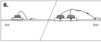
Ensure insulation do not abut and cover the luminaire\*.
