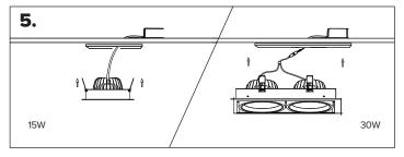
Fold mounting clips up to the sides of the luminaire and insert luminaire through the cut-out.
