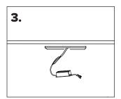
Insert driver and cables through the cut-out into the ceiling cavity and plug into a pre-wired socket outlet inside the ceiling.
