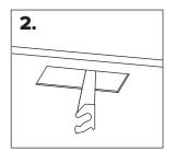
Cut an appropriately sized hole in the ceiling, matching the specified cutout dimensions for your model.
